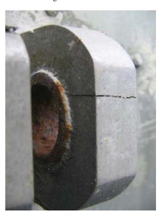
Example: Carbon steel bushing (not SSI) corrodes and causes the fitting (SSI) to crack. Early detection of corrosion and replacement of the bushing would have prevented the lug from failing.
